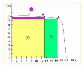
**Schematic Diagram:** Picture 2 shows typical 12V battery solar charge system V-A curve.
