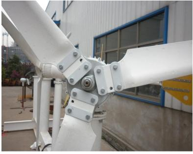
4. Assemble the nose cone by screw
