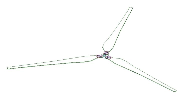
Adjusting the distance between each tip of the blades to equal, making sure LI=L2=L3( allowable difference ±5 mm)
