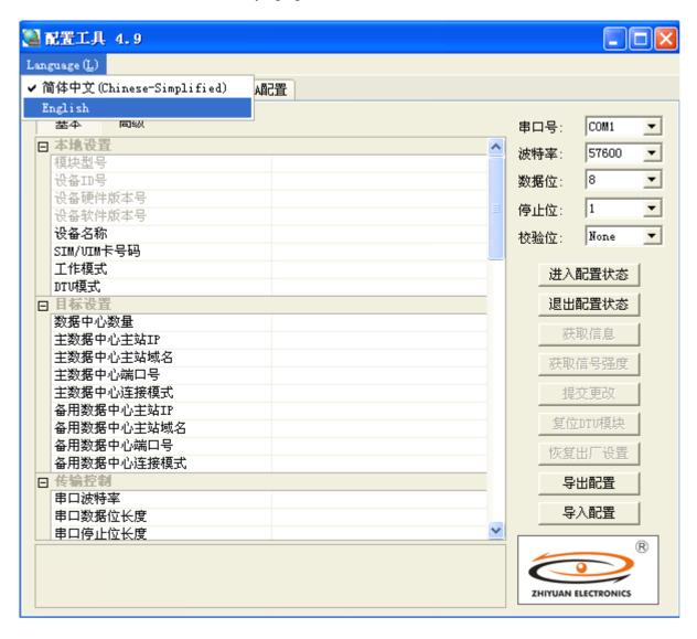
Clicking "abtain information" to get the configuration of GPRS, then switching into advanced mode, drugging down to the screen to find the name of APN, changing the name into the one provided by SIM card supplier. If password needed, finding the reference from SIM card supplier and filling information in the corresponding place.
