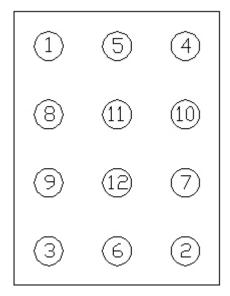
Torque spanner is required for fastening the bolts.( torque requirement:  $60\pm2$ )
