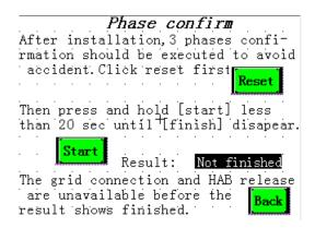
If the phase sequence can not be confirmed, exchanging the connecting sequence of cable A.B.C between grid and controller, then confirming again of the phase sequence.
