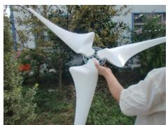
4. Blades installation: installed the blades on the dowel disc onto the generator shaft;
