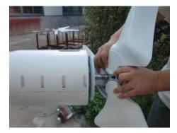
5. Put the bolt onto the dowel disc groove and connect it with the generator shaft, Fasten it with spanner and rotate the blades clockwisely at the same time;
