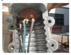
Please install the rubber ring onto the tower and complete the other cover(Note: the rubber ring should be instal ed inside the groove);
