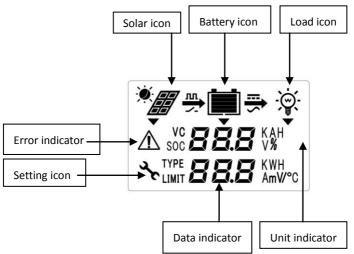
The two LED indicators above the LCD show that battery is charging, and a red indicates error conditions.
