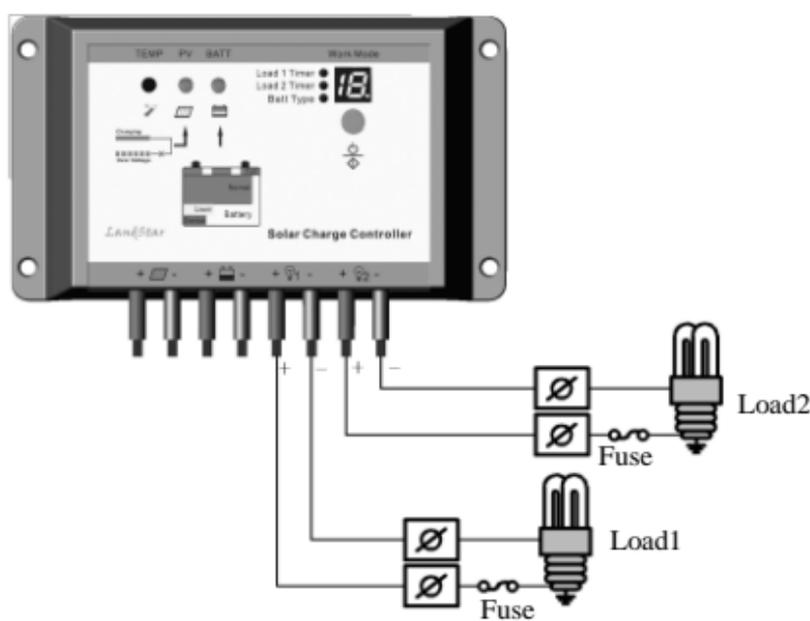
Figure 3-3 Load Wiring
