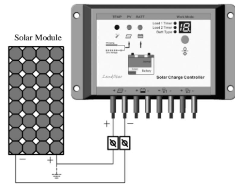
Figure 3-4 Solar wiring
