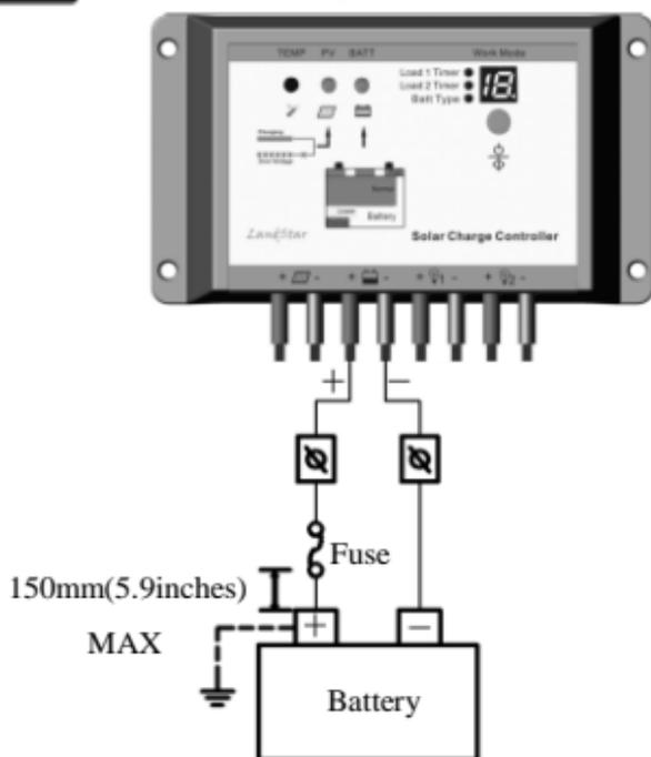
Figure 3-2 Battery connecting
