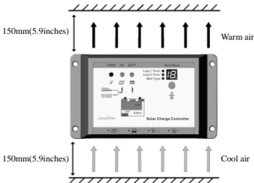
Figure 3-1 Mounting and cooling
