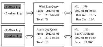
Press OK to enter the monitoring interface when the inverse cursor point to monitor item. Press ESC button to exit. Work Log and Alarm Log could be browsed in this interface, the operation is as follows:
