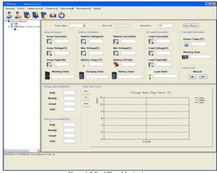
Figure 6-2 Real Time Monitoring
