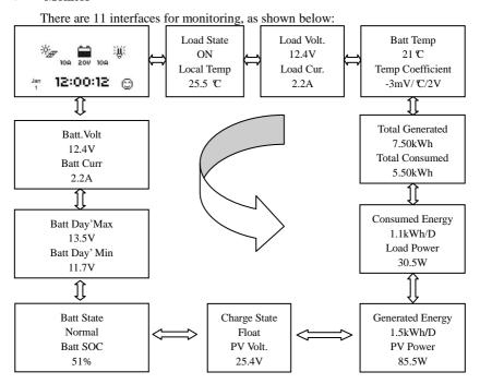
Press OK to enter the monitoring interface when the inverse cursor point to monitor item.
