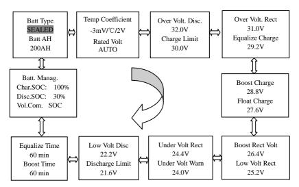
You should input the user password(see above) before setting the parameters. In setting mode, all the parameters can be modified. And will immediately effect when saved. The detail and value range of control parameter are shown in the tables below:
