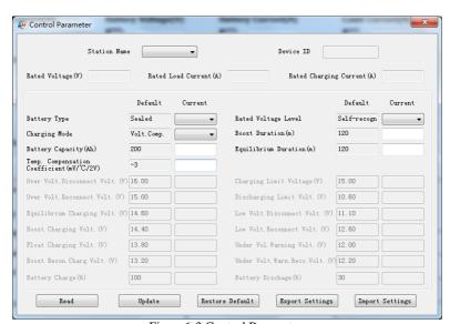
Figure 6-3 Control Parameter Load Configuration Device ID Station Name Load Control Mode Manually On By Default Manually Off By Default Timing Control Turn-On Time1 17:16:39 Turn-Off Time1 17:16:39 Turn-On Time2 17:16:39 Turn-Off Time2 17:16:39 5.00 Light On Turn-On Volt. (V) Delay(m) Turn-Off Volt. (V) 6.00 Delay(m) Light On + Time Work Time1 02:00 Work Time2 02:00 10 🚔 : Night Time (h) Read Update Import Settings Export Settings
