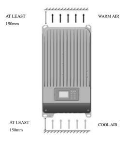
Figure 3-1 Required mounting clearance for air
