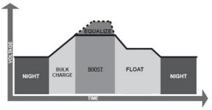
Figura4-2 iTracer charging algorithm
